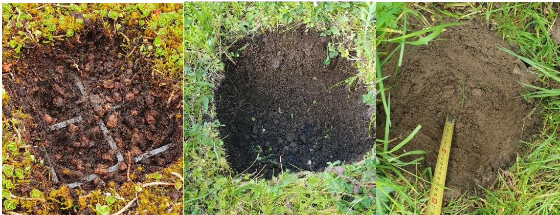
Figure 12: monolith for macrofauna sampling (left: extensive roof, 4cm-depth; middle: semi-intensive roof, 15cm depth; right: intensive roof, 20cm depth) (©Nolwen Levallant 2023)
